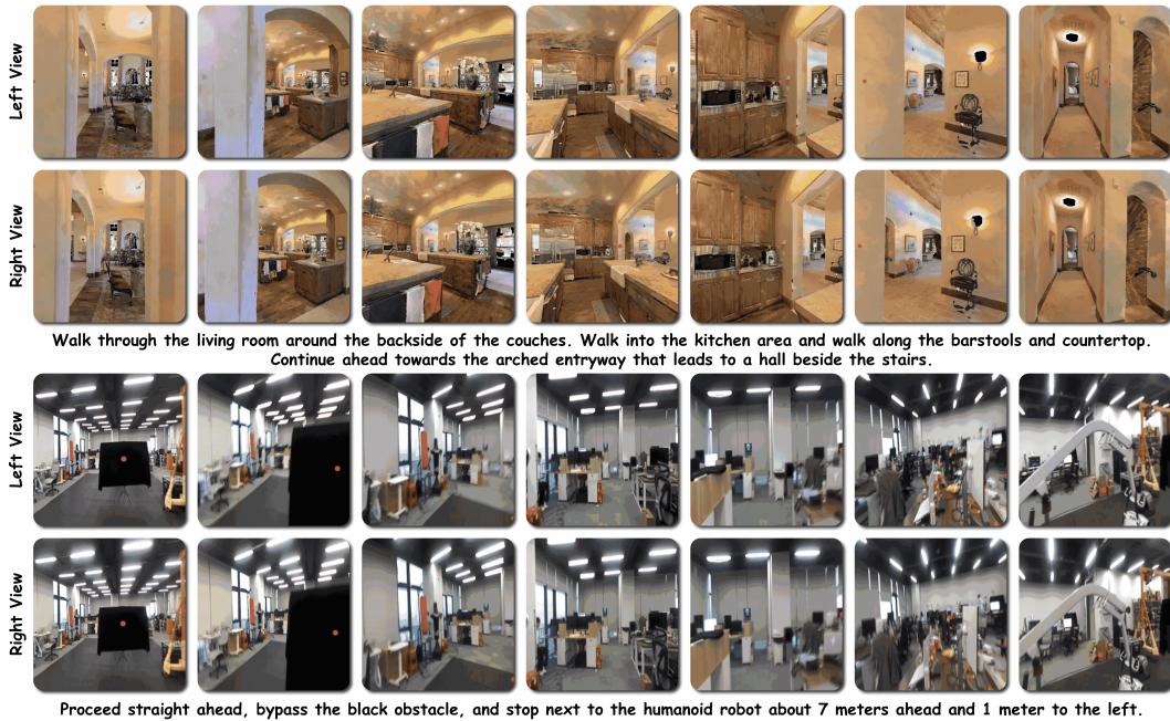
Figure 10: First-person stereo observations in simulation and real-world deployment. (a) Top: First-person left- and right-view observations from a representative virtual environment, where the rendered target-location prior provides persistent visual guidance during navigation. (b) Bottom: First-person left- and right-view observations from a representative real-world Gym scenario, demonstrating the deployment of StereoNav on the Unitree G1 robot under physical navigation conditions.
